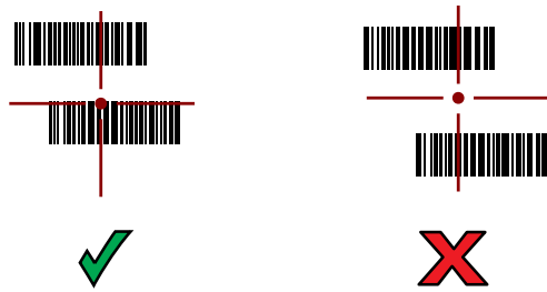
Figure 18 RS6000 Pick List Mode with Multiple Barcodes in Aiming Pattern
