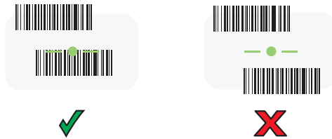
Figure 46 RS6000 Pick List Mode with Multiple Barcodes in Aiming Pattern
